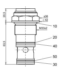
Cavity drawing according to ISO 7789–33–06–0–98
