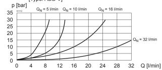
Q = f (s, x) Volume flow adjustment characteristics ( $\Delta p$  = 10 bar) [Type: ADB-V]
