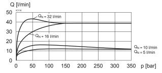
$\Delta p = f(Q)$  Pressure loss/flow characteristics (s = 100 %) [Types: ACB-S]
