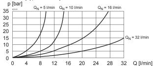
Q = f (s, x) Volume flow adjustment characteristics ( $\Delta p$  = 10 bar) [Types: ACB-S]
