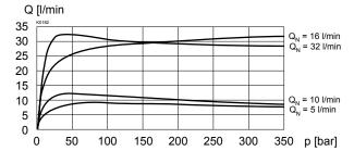
Pressure loss/flow characteristics (s = 100 %)  $\Delta p = f(Q)$ [Type: ACB-S]
