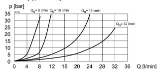
Q = f (s, x) Volume flow-signal-characteristics ( $\Delta p$  = 10 bar) [Type: ACB-S]
