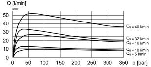
$\Delta p = f(Q)$ Pressure loss/flow characteristics (s = 100 %) [Type: ADB-V]
