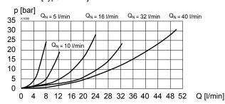
Q = f (s, x) Volume flow-signal-characteristics ( $\Delta p$  = 10 bar) [Type: ADB-V] (s corresponds to preset value signal and x corresponds to spool stroke)
