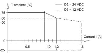
If mounted on the solenoid  $\square$  60/12V the current has to be limited to 1.8 A, otherwise the proportional-amplifier could be overloaded.
