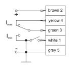
Connection with external power source release/block with PLC, PC or NC
