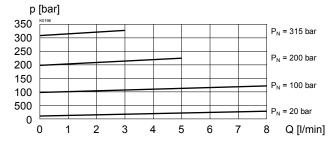
p = f(I) Pressure adjustment characteristics (Q = 1 I/min)
