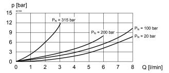
Q<sub>I</sub> = f (p) Leakage volume flow characteristics
