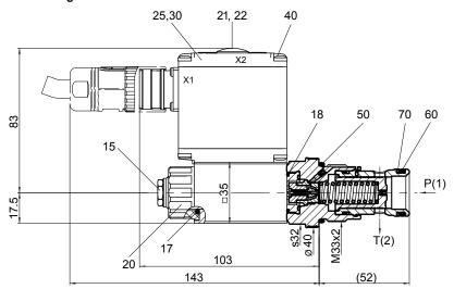
Cavity drawing according to ISO 7789–33–02–0–98
