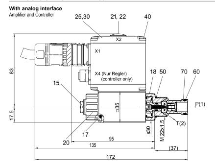
Cavity drawing according to ISO 7789-22-02-0-98
