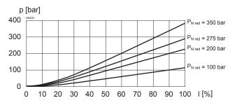
$p_{red}$  = f (Q) Pressure volume flow characteristics (Minimal adjustable pressure)
