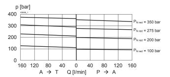
$p_{red} = f(I)$ Pressure adjustment characteristics [at Q = 0 l/min (static)]
